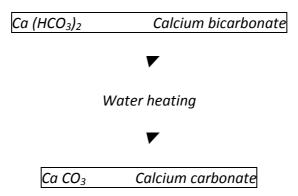
As calcium carbonate - scale – can be formed only starting from calcium bicarbonate (as simplified in the previous scheme), if we separate this latter (IONISATION) deposits and incrustations can be avoided (carbonates).
